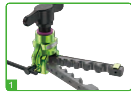
1 The expansion strip is inserted into the expansion body
