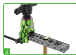
2 The copper pipe enters the hole, and the limit plate is on the copper pipe
