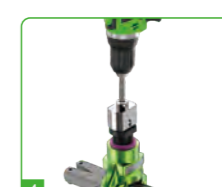
4 Or use cordless drill for fast flaring
