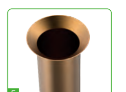
5 Finalize of expanding 45° copper pipe
