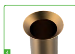
4 Complete expanding 45° copper pipe
