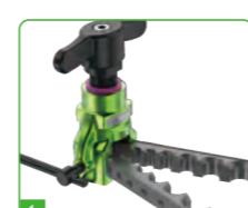
1 The expansion strip is inserted into the expansion body
