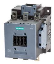
Contactor 110...127 V AC/DC AC3 kW 400 V AC (50...60 Hz) / DC operation auxiliary contacts 2 NO + 2 NC, 3-pole, size S6 bar connections conventional operating mechan. screw terminal
