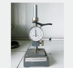
Thickness Testing Instrument
