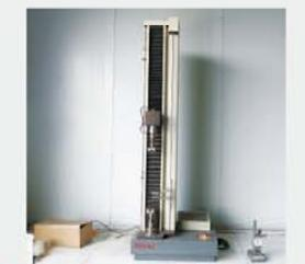
Rubber Tensile Testing Instrument
