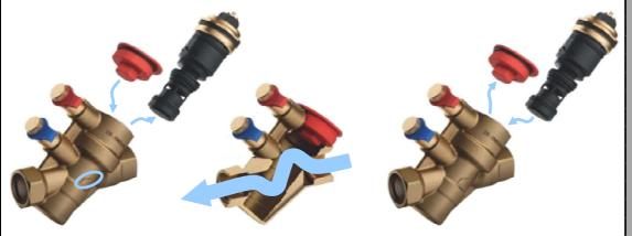
It is possible, at any time and even after the installation of the valve onto the line, to install onto the VIR Fig. 9705B valve a linear Vaurien-B actuator (for more information please refer to its specific technical sheet).
