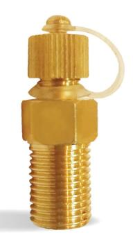
ANBI Test Plugs provide an economical solution to installing pressure and temperature gauges in chilled water systems. The unique "Dual Core" design allows for the bottom seal to close, sealing the system before the probe is fully removed through the top core.
